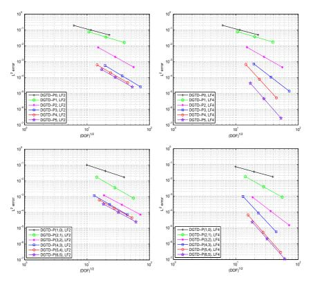
Figure 3: Problem 1: *h*-convergence of the DGTD- $\mathbb{P}_p$  (top) and DGTD- $\mathbb{P}_{(p_1,p_2)}$  (bottom) methods using the LF<sub>2</sub> (left) and LF<sub>4</sub> (right) schemes.  $L^2$  error at time T = 2 as a function of the square root of #DOF.
