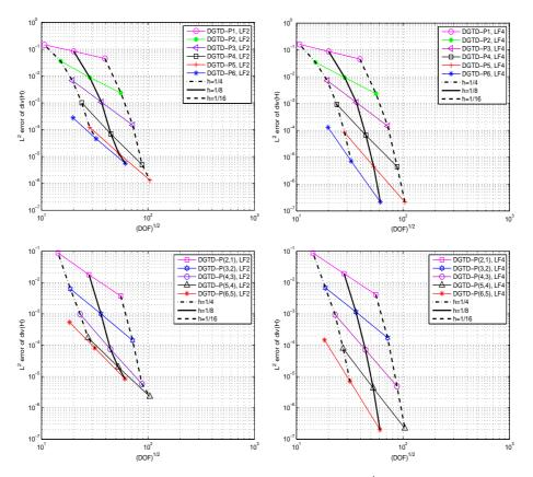
Figure 6: Problem 1: *h*- and *p*-convergence of the divergence of  $\vec{H}$ . DGTD- $\mathbb{P}_p$  (top) and DGTD- $\mathbb{P}_{(p_1,p_2)}$  (bottom) methods using the LF<sub>2</sub> (left) and LF<sub>4</sub> (right) schemes. Errors evaluated at time T = 2.
