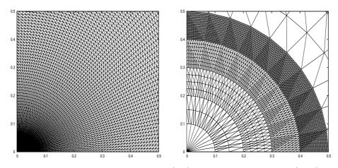
Figure 9: Problem 2: Conforming mesh (left) and non-conforming mesh (right).
