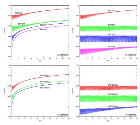
Figure 2: Problem 1: Time evolution of the  $L^2$  error. DGTD- $\mathbb{P}_p$  (top) and DGTD- $\mathbb{P}_{(p_1,p_2)}$  (bottom) methods using the LF<sub>2</sub> (left) and LF<sub>4</sub> (right) schemes.
