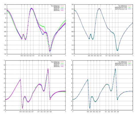
Figure 10: Problem 2: 1D distribution of the  $E_z$  (top) and  $H_y$  (bottom) components along y = 0.0 at time T = 5. Conforming DGTD- $\mathbb{P}_p$  method (left) and non-conforming DGTD- $\mathbb{P}_{p_i}$  method (right).
