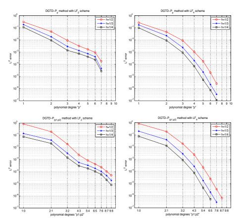
Figure 4: Problem 1: *p*-convergence of the DGTD- $\mathbb{P}_p$  (top) and DGTD- $\mathbb{P}_{(p_1,p_2)}$  (bottom) methods using the LF<sub>2</sub> (left) and LF<sub>4</sub> (right) schemes.  $L^2$  error at time T = 2 as a function of the approximation order *p*.
